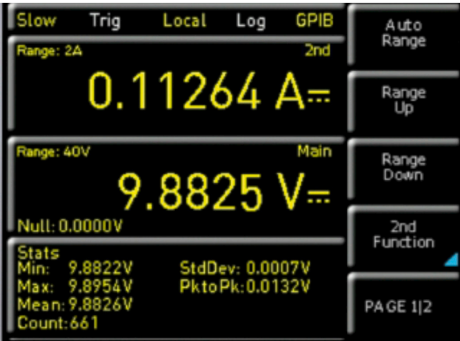
Simultaneous measurement display: Simultaneous display of three measurements, including DCI and ACI at the same time
