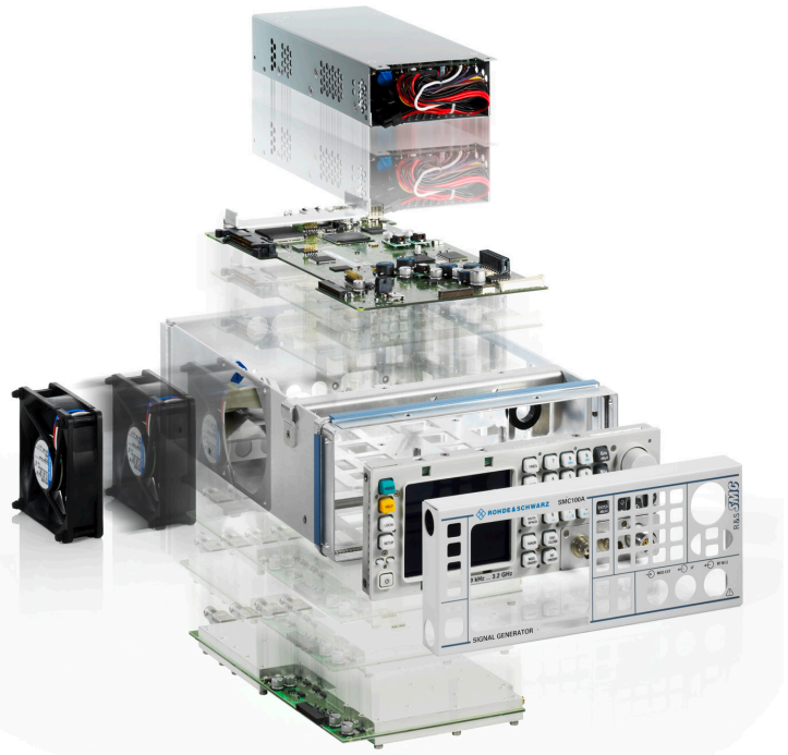
Minimized total cost of ownership: A minimum of modules in the R&S®SMC100A means high reliability and easy servicing
