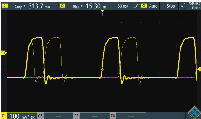
The high-speed acquisition system of the R&S®ScopeRider captures up to 50 000 waveforms/s and uncovers rare and unexpected signal anomalies
